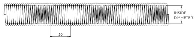
Inside Spring Diameters can be: 51mm,67mm, 95mm, 152mm.
